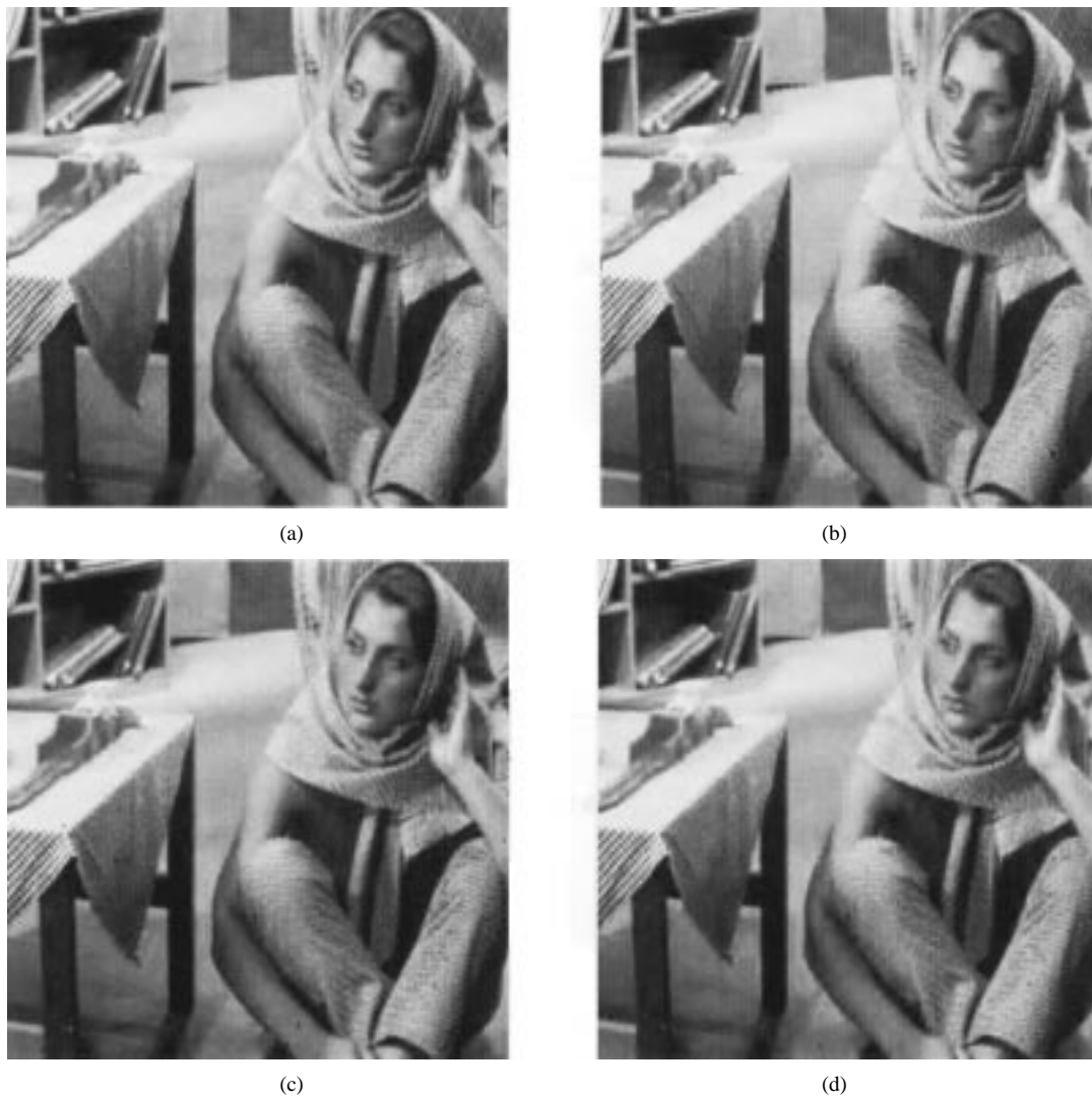
Fig. 5. Coding results of Barbara at 1:32 compression ratio. (a) SPIHT, 9/7-tap biorthogonal wavelet. (b) Embedded 8 \times 8 DCT. (c) Embedded 8 \times 16 GLBT. (d) Embedded 8 \times 24 LILT.
