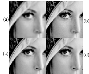
Fig. 6. Comparison of various methods for S = 1/2 . (a) Our method with N = 2 , C_I = 2 , C_O = 4 , PSNR = 28.75 dB, Multiplications Per Pixel (MPP) = 0.13. (b) Method of [5], PSNR = 34.69 dB, MPP 1.25. (c) Our method with N = 5 , C_I = 5 , C_O = 8 , PSNR = 35.34 dB, MPP = 1.41. (d) Spatial domain PSNR = 30.33 dB, MPP = 3.44.
