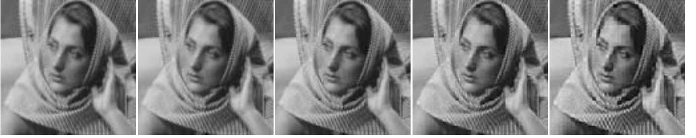
Fig. 8. Pre-filtering's block-wise flattening effect with 8 \times 8 block size. From left to right: original image; after 2-point pre-filtering (borrowing 1 sample at each boundary); after 4-point pre-filtering (borrowing 2 samples); after 6-point pre-filtering (borrowing 3 samples); after 8-point pre-filtering (borrowing 4 samples).
