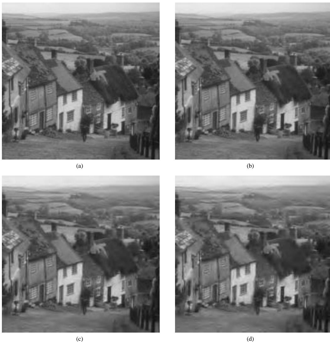
FIGURE 8. Goldhill coded by the 8 \times 40 GenLOT coder at (a) 1:16, 33.36 dB (b) 1:32, 30.79 dB (c) 1:64, 28.60 dB (d) 1:100, 27.40 dB.
