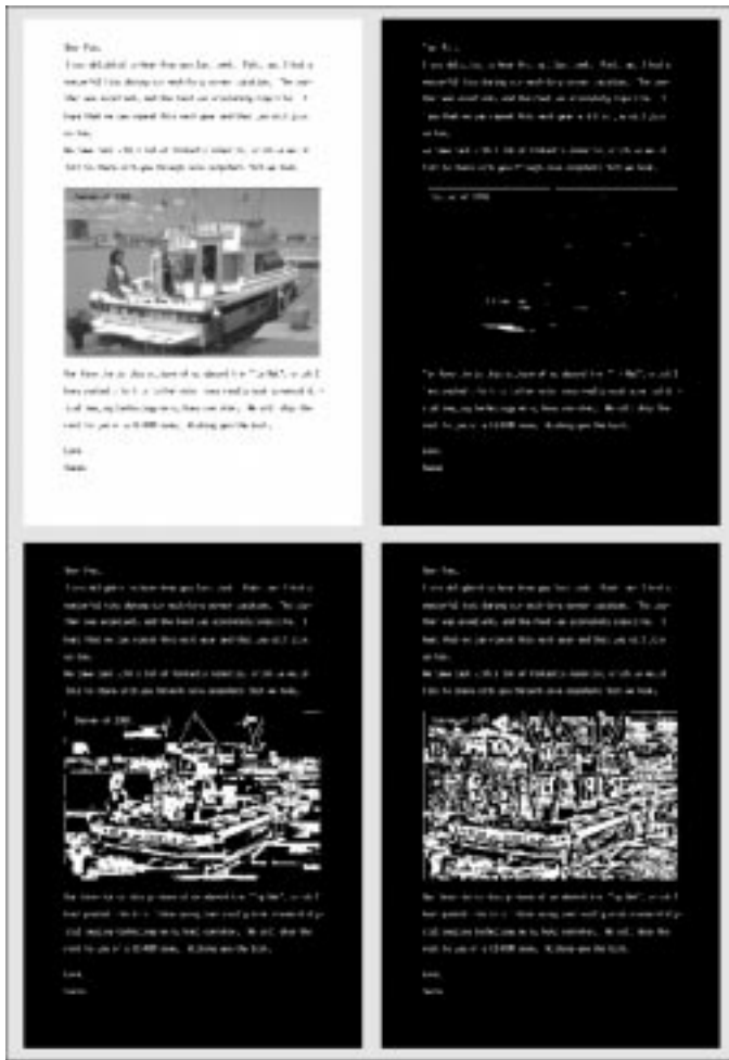
Fig. 6. Mask examples for image “compound1”: top left, original image; top right, mask for minimum \lambda ; bottom left, same for intermediary \lambda ; bottom right: same for maximum \lambda .
