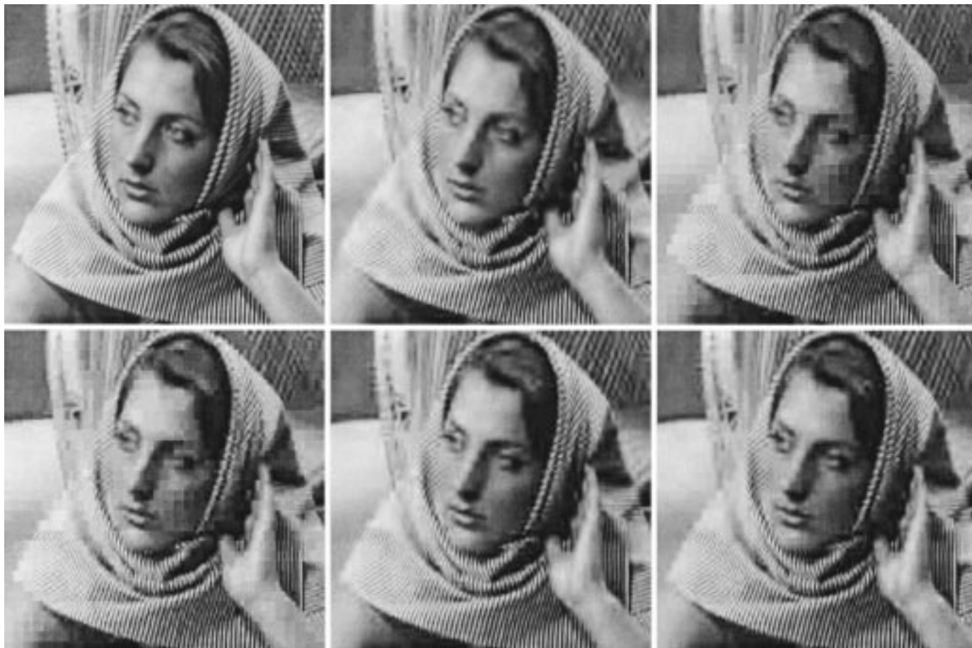
Fig. 19. Enlarged 256 \times 256 Barbara portions at 32:1 compression ratio. Top row, from left to right: original image; coded by 9/7-tap wavelet, 27.58 dB; coded by 8 \times 8 DCT, 27.28 dB. Bottom row, from left to right: coded by 8 \times 8 binDCT, 27.25 dB; coded by 8 \times 16 LiftLT-I, 28.93 dB; coded by 8 \times 16 LiftLT-II, 28.49 dB.
