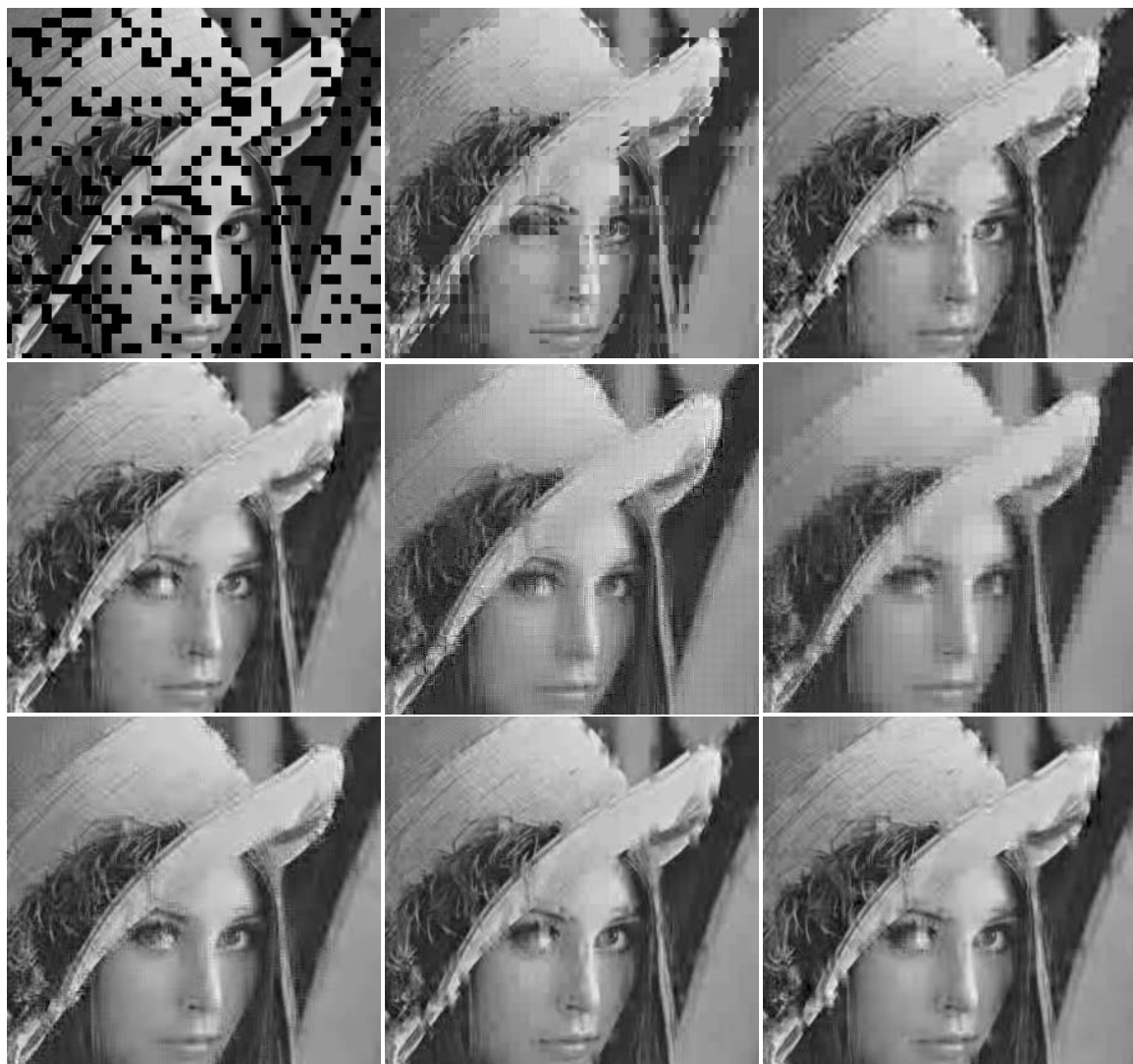
Fig. 7. Portions of reconstructed Lena image (coded at 0.25 bpp), suffering from 25% random loss. From left to right, top row: locations of loss; DCT (25.71 dB); LOT opt (25.82 dB); middle row: LT opt (25.73 dB); T9 (24.82 dB); P1 (25.96 dB); bottom row: P2 (27.13 dB); P3 (26.67 dB); P4 (25.89 dB).
