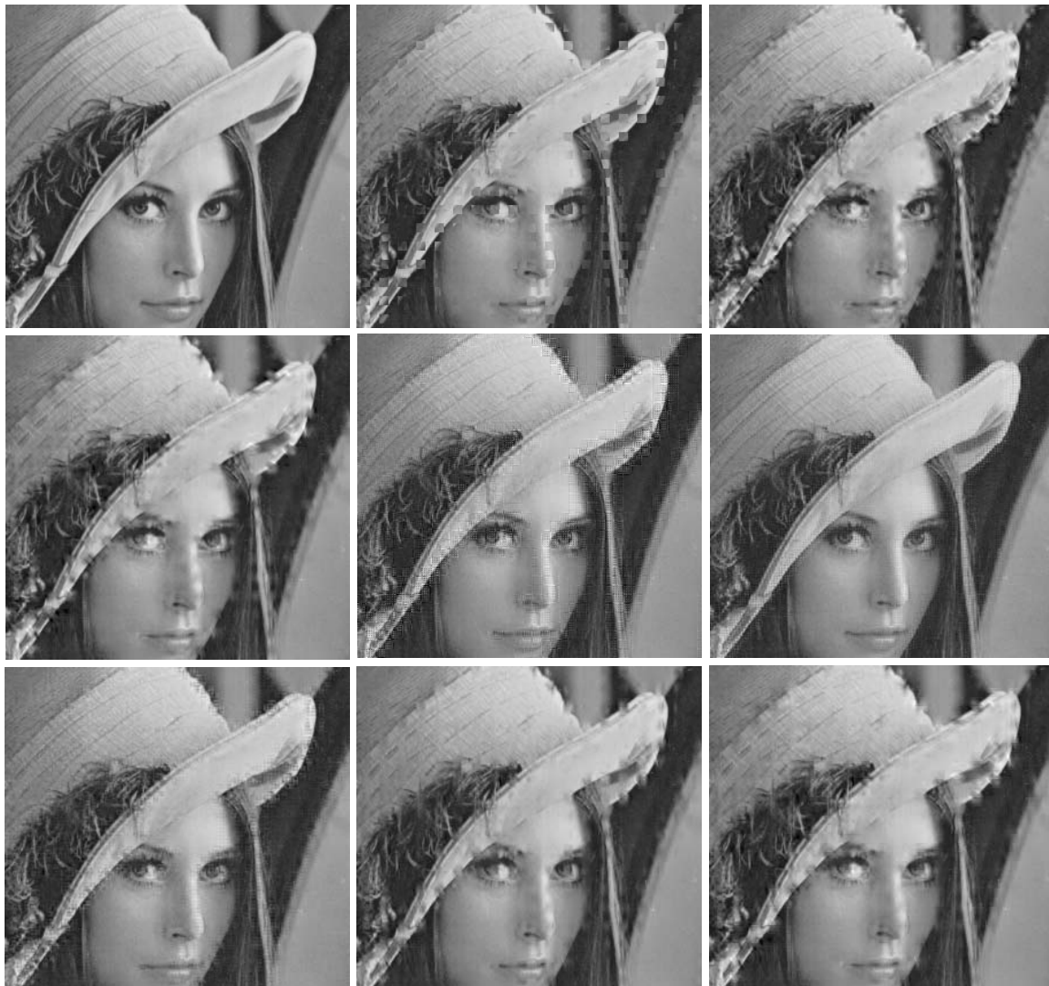
Fig. 6. Portions of reconstructed Lena image without quantization, suffering from 25% regular loss. From left to right, top row: original; DCT (27.41 dB); LOT opt (27.42 dB); middle row: LT opt (27.07 dB); T9 (27.30 dB); P1 (30.88 dB); bottom row: P2 (29.79 dB); P3 (28.57 dB); P4 (27.15 dB).
