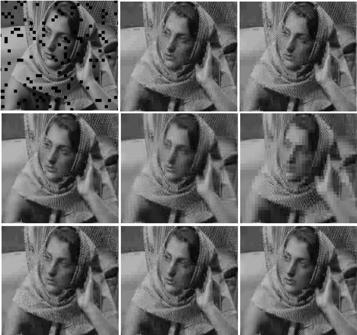
Fig. 8. Portions of reconstructed Barbara image (coded at 1 bpp), suffering from 10% random loss. From left to right, top row: locations of loss; DCT (29.69 dB); LOT opt (29.61 dB); middle row: LT opt (29.47 dB); T9 (28.29 dB); P1 (28.62 dB); bottom row: P2 (29.45 dB); P3 (30.05 dB); P4 (29.55 dB).
