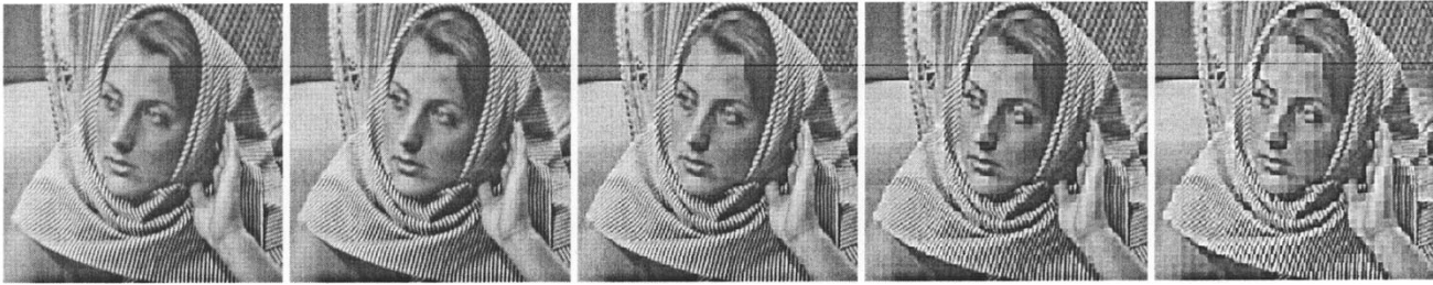
Fig. 8. Pre-filtering's block-wise flattening effect with 8 \times 8 block size. From left to right: Original image; after two-point pre-filtering (borrowing one sample at each boundary); after four-point pre-filtering (borrowing two samples); after six-point pre-filtering (borrowing three samples); after eight-point pre-filtering (borrowing four samples).
