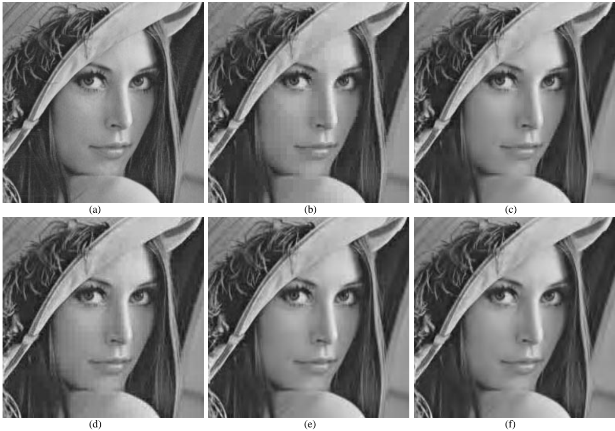
Figure 56: Perceptual comparison between various transforms at 1:32 compression ratio. Enlarged portions. (a) Original Lena image. (b) 8 \times 8 DCT. (c) 2 \times 24 \ 6 \times 8 VLGLBT. (d) 8 \times 16 LOT. (e) 8 \times 16 GLBT. (f) 9/7-tap wavelet.
