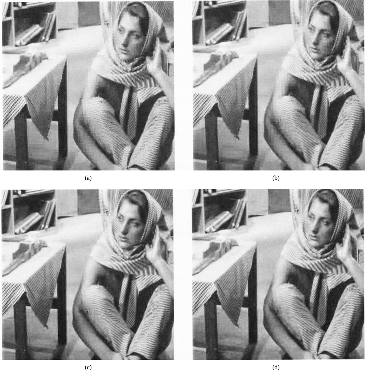
Fig. 12. The 512 \times 512 Barbara image coded at 1:32 using various transforms: (a) 8 \times 8 DCT, (b) 8 \times 16 LOT, (c) 8 \times 16 GLBT, and (d) 16 \times 32 GLBT.
